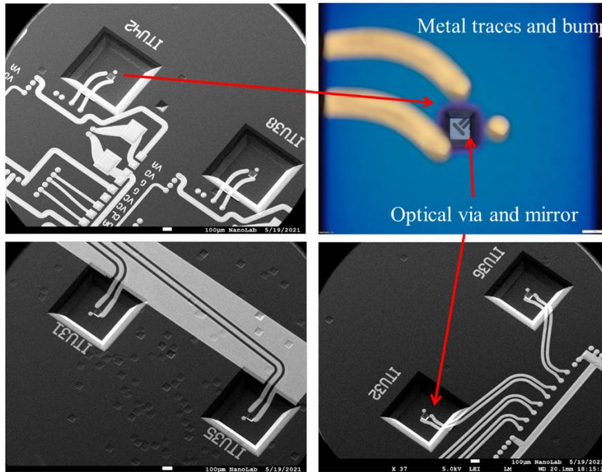
Figure 18. Optical and SEM images of processed back side of PIC.
