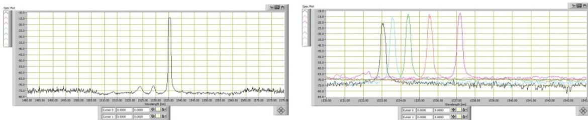
Figure 13. (Left) Spectrum and SMSR of VCSE; (Right) Wavelength tuning.
