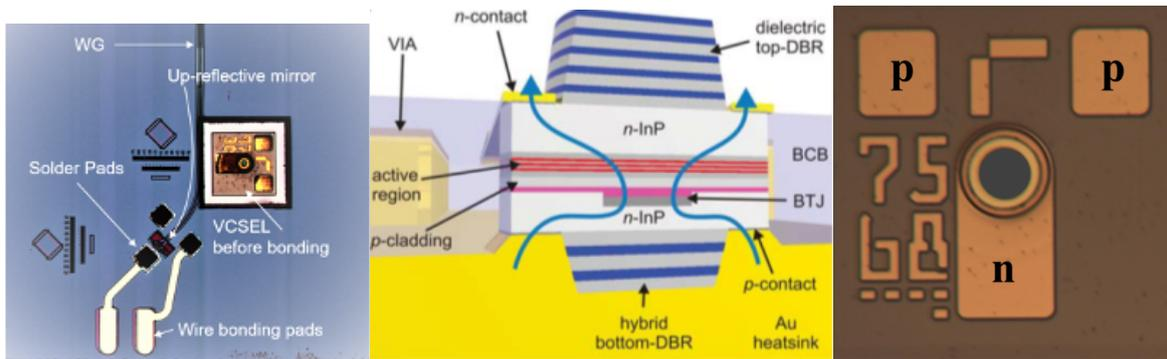
Figure 15. VCSEL top circular mirror (on the left), short cavity VCSEL structure (center) and chip layout (on the right).
