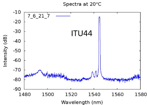
Figure 37 Tx MOD1-R3C5 output spectrum after the fibre pigtail at ITU channel 44.
