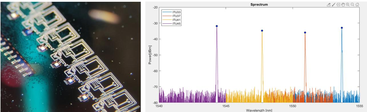
Figure 20. Image of back side of SiPh PIC with embedded VCSELS (Left); Spectrum of 4 VCSELS as captured at the output of the SiPh PIC multiplexer (Right).
