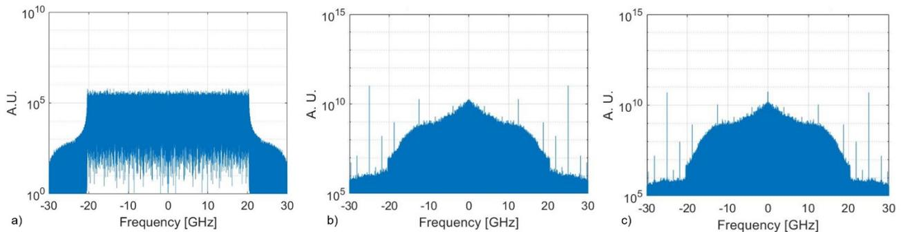
Figure 31 Electrical spectrum of a) DSB TX signal; b) RX signal of DSB-modulated VCSEL for 44 dB OSNR. c) RX signal of SSB-modulated VCSEL for 44 dB OSNR.
