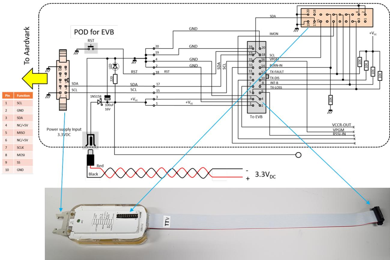
Figure 9. Utility box POD 2 for I2C to Aardvark computer interfacing and to EVB.
