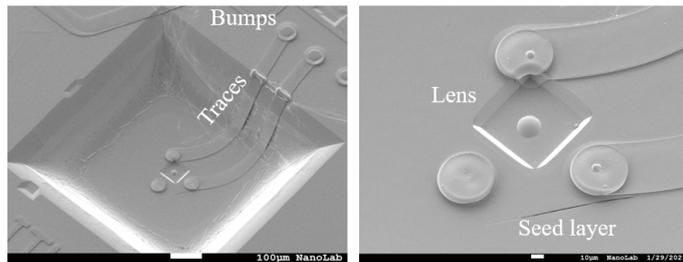
Figure 24. SEM photos before removing the plating seed layer: fabricated cavities for the single VCSEL (left). Zoom-in photo of small cavity and lens and pads for VCSELS (Right).
