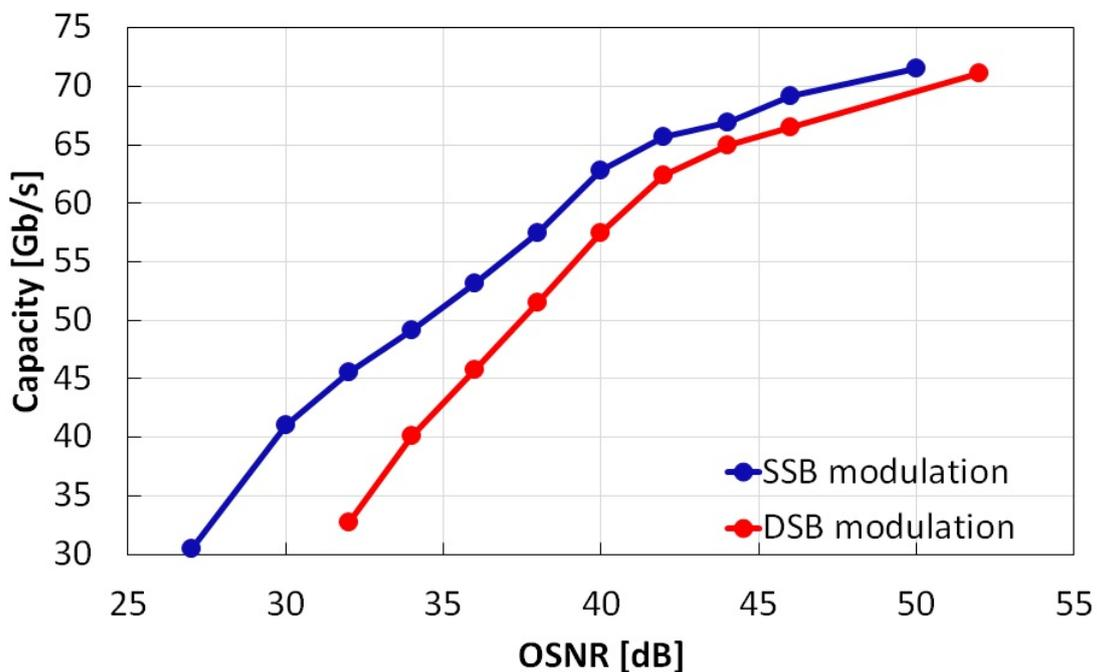
Figure 30. Measured capacities at the output of the single-channel transmitter for DSB and SSB modulations.
