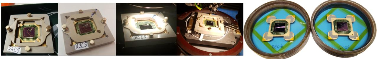
Figure 10. All manufactured MODs under their assembly jigs.
