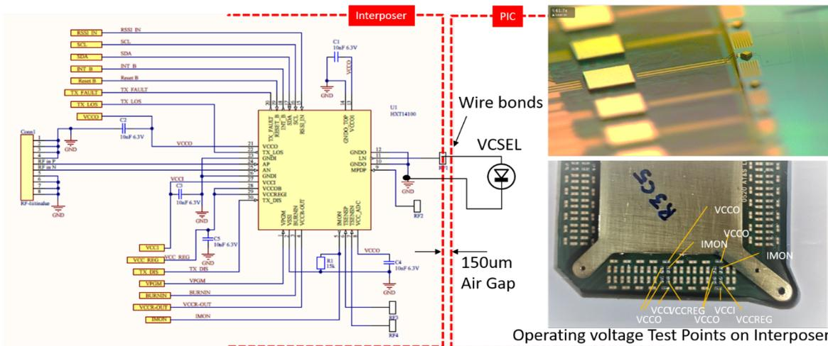
Figure 7 HXT14100 VCSEL Driver Electrical diagram on the Tx MOD.
