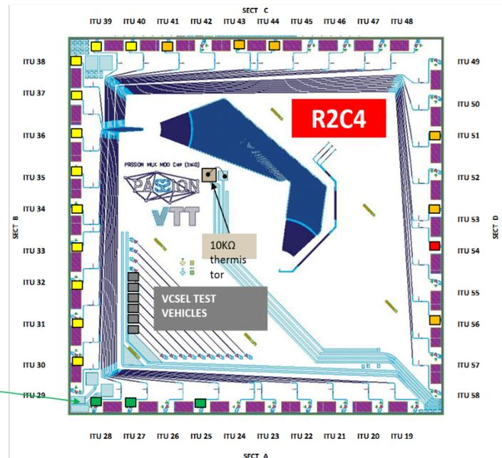
Figure 11. MOD MPW9-R3C3 VCSEL and ITU channel map.
