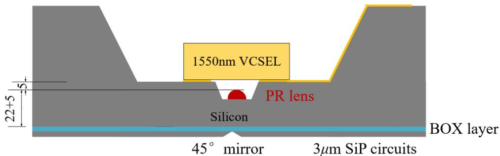
Figure 21. Integration scheme of VCSELS and down reflecting mirrors including PR lens.
