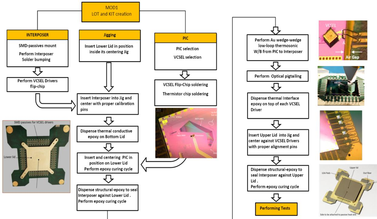
Figure 1. MOD simplified assembly flow chart.
