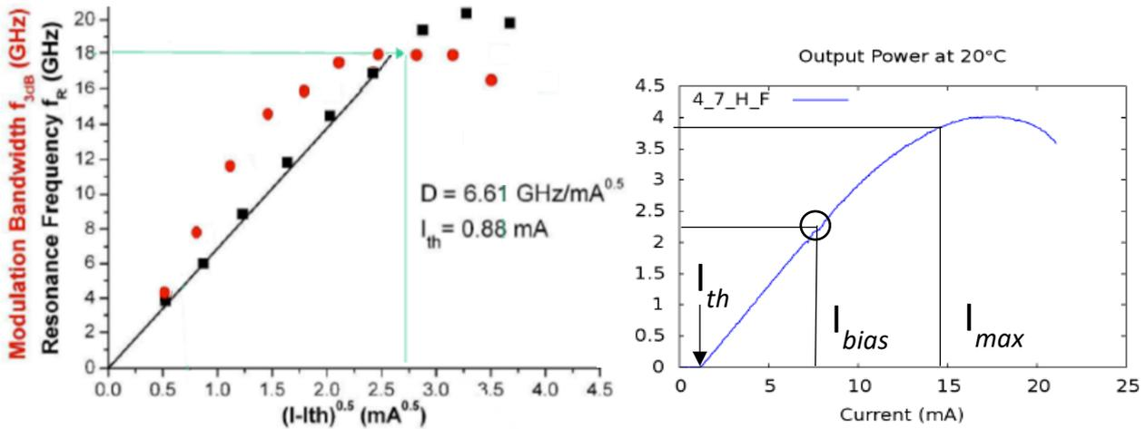
Figure 12. Modulation bandwidth (red circle) and resonance frequency (black square) as a function of the  $I_{bias}$ . Maximum bandwidth is achieved at  $I_{bias}$  of about 8.5mA, corresponding to  $(I - I_{th})^{0.5} = 2.74$  (having  $I_{th} = 1$  mA).
