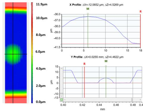
Figure 25. Measured 3D map for the lens in the small cavity, both x- and y- profile indicate the height of the micro lens is 4.5  $\mu\text{m}$  and radius of curvature is 10.9  $\mu\text{m}$ .
