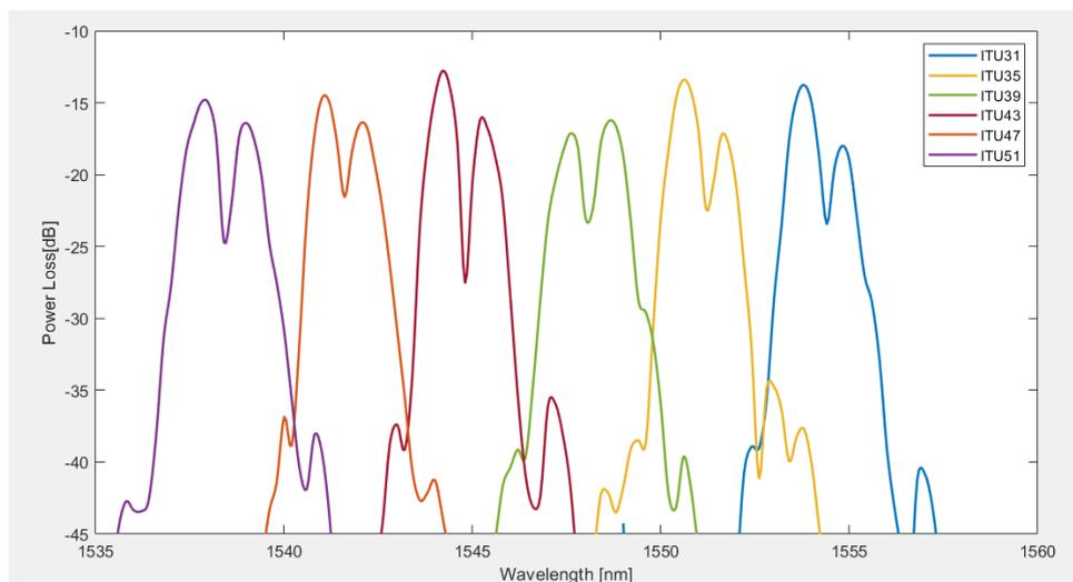
Figure 19. Measured optical losses for light injected via a lensed fiber into a channel input and measured at the multiplexed output.
