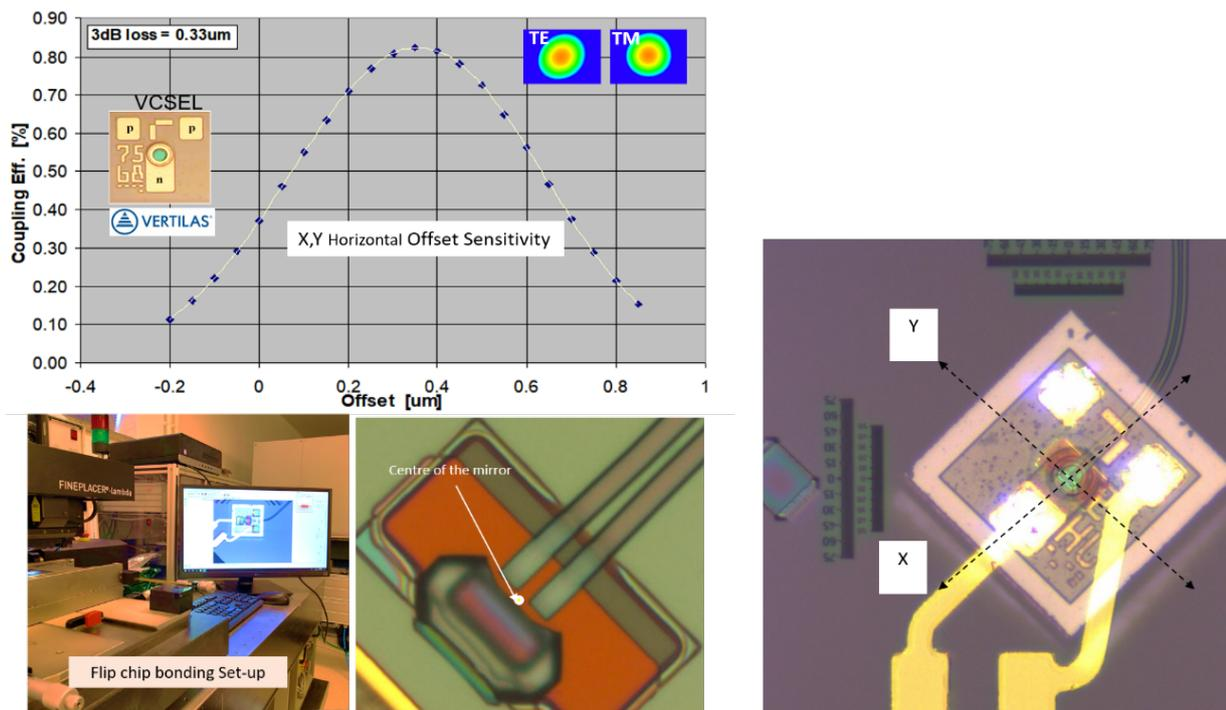
Figure 16 VCSEL alignment sensitivity during Flip-Chip bonding.
