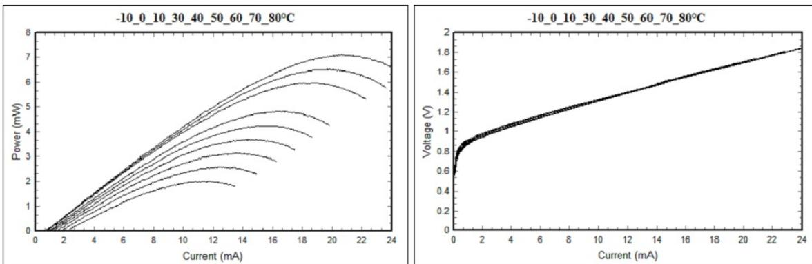
Figure 14. (Left) LI graphs from -10°C to 80°C; (Right) VI graph.
