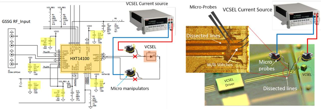
Figure 35 (Right) Probing VCSELs on the Tx MOD with external probes and precision current source . (Left) Insulating driver from VCSEL with dissected GSG lines, close to wirebonds.
