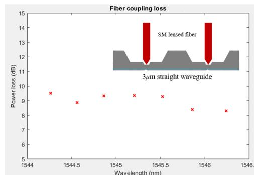
Figure 26. calibration measurement in the VCSEL tuning range by using two lensed fibers. Insert: test scheme shows two vertically aligned lensed fibers and mirror on both sides of the straight waveguide.
