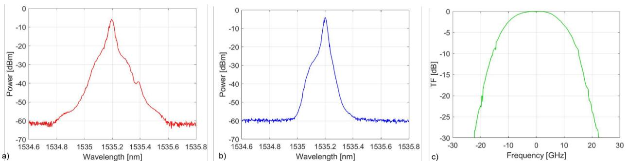
Figure 32 Optical spectrum of a) DSB-modulated VCSEL; b) SSB-modulated VCSEL for 44 dB OSNR. c) Transfer function of the 25-GHz WSS, as emulated by the Finisar Waveshaper.
