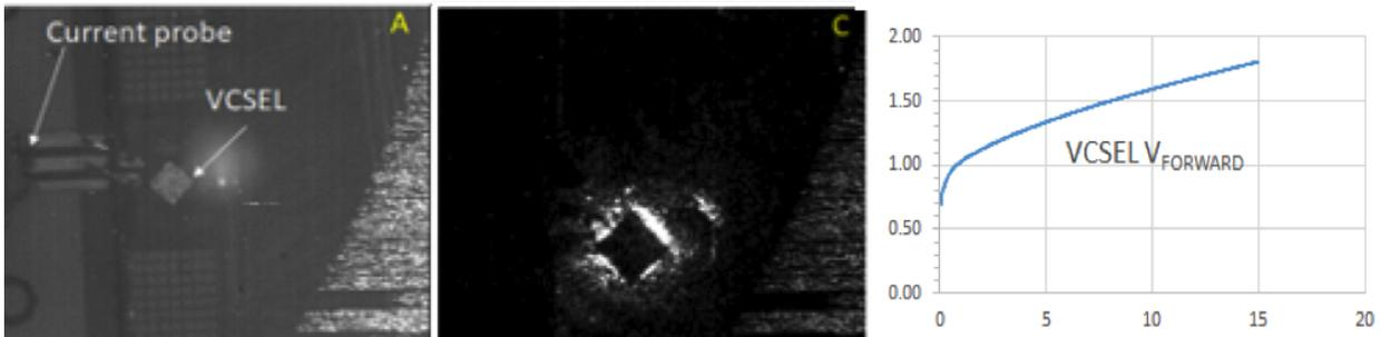
Figure 36 Probed VCSEL, IR light scattered, measured VCSEL voltage.
