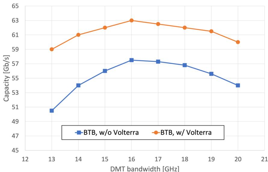
Figure 34. Multi-channel transmitter output capacities in function of DMT electrical bandwidth with (orange circles) and without (blue squares) Volterra equalization with 25-GHz channel spacing.
