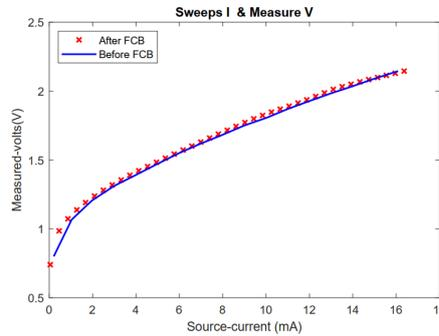
Figure 27. IV curve of the VCSEL before and after bonding.
