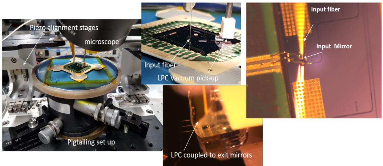
Figure 3. (Left) Pigtailling bench set up and (Centre to Right) Lensed Input fiber and LPC pigtailling.
