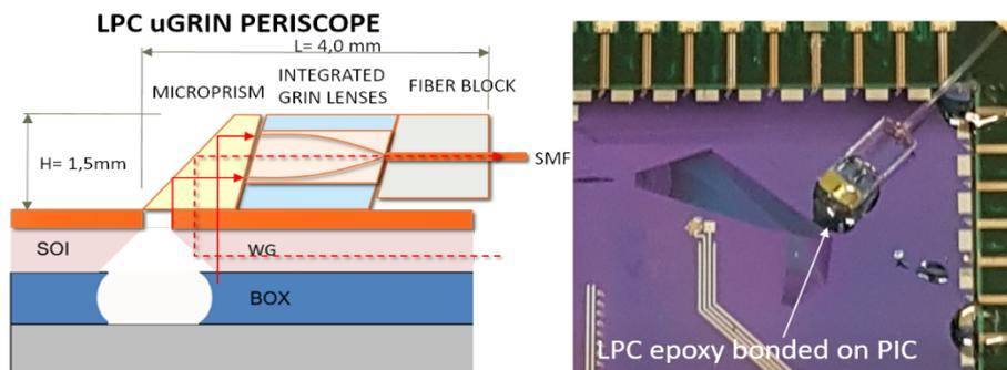
Figure 2. LPC design and LPC coupled to PIC exit mirror.
