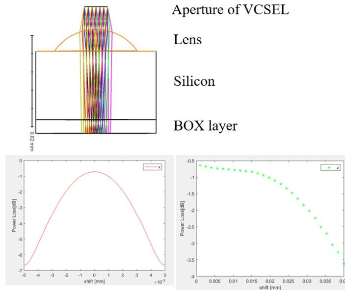
Figure 22. Zemax simulation results for light coupling between VCSEL and Silicon waveguide with the help of a PR lens.
