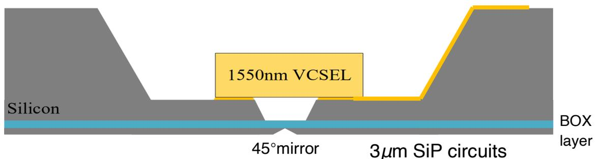
Figure 17. VCSEL assembly concept by embedding in cavity in back side of PIC.
