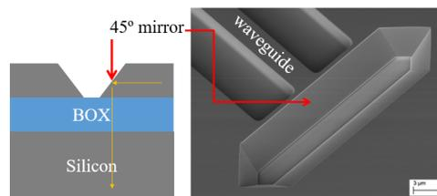
Figure 23. schematic drawing (left) and SEM photo of waveguide and TIR mirror. The yellow arrow indicates the light path.
