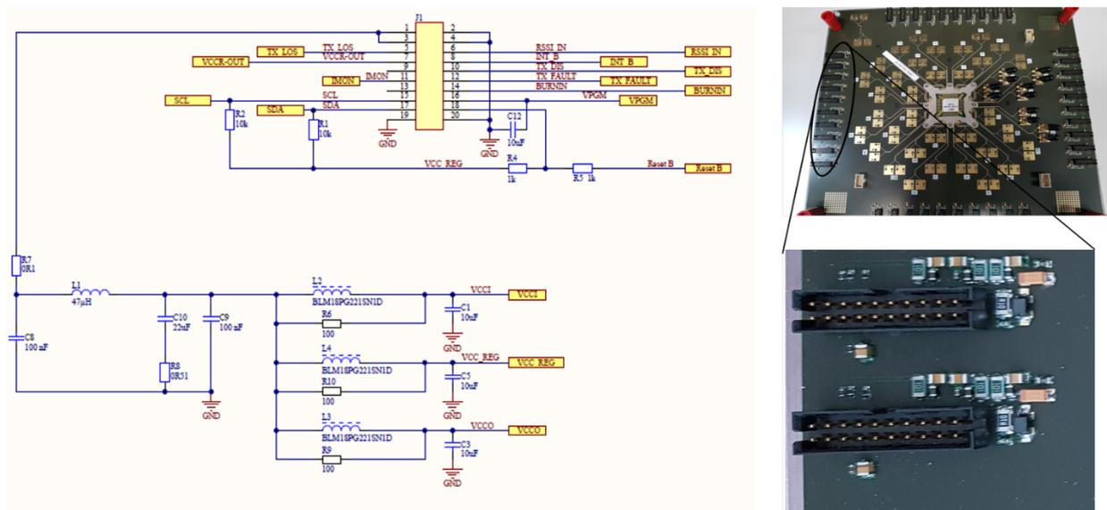
Figure 8. EVB Channel connector to address all needed power supplies and I2C control interface to a corresponding VCSEL driver on MOD1. On EVB there are up to 40 independent channel connectors.
