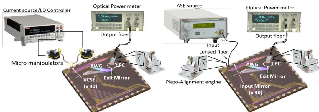
Figure 4. PIC to fibre alignment strategy. (Left) Power-up any VCSEL on PIC with micro-manipulator probes or (Right) launching light with a broadband source (eg.80nm) to any available input mirror through a lensed fibre matching the 2.8μm MFD of the SOI waveguide.
