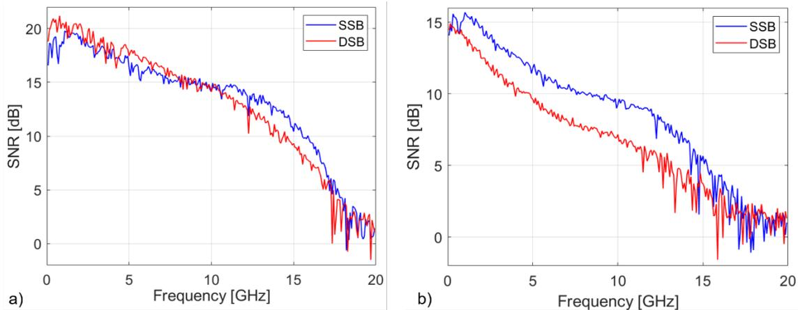
Figure 33. SNR profiles of SSB-modulated (blue curve) and DSB-modulated (red curve) VCSEL for: a) 44-dB OSNR; b) 32-dB OSNR.
