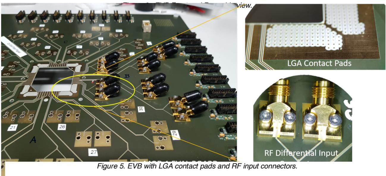
Figure 5. EVB with LGA contact pads and RF input connectors.
