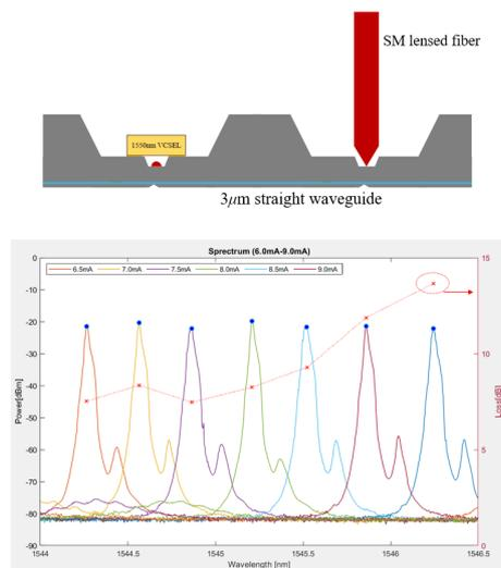
Figure 28. Spectrum measurement after VCSEL bonding. The calculated power loss of the lens system.
