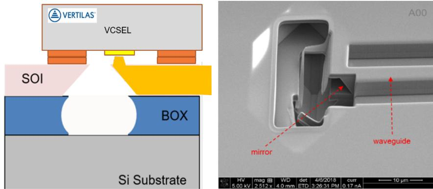
Figure 9 (Left) A schematic view of an internal up-reflecting mirror at the end of the  $3\mu\text{m}$  waveguide. Light is totally internally reflected at the 45 degree tilted end facet of the waveguide. (Right) SEM image with TIR mirror plane exposed (using ion beam etching).
