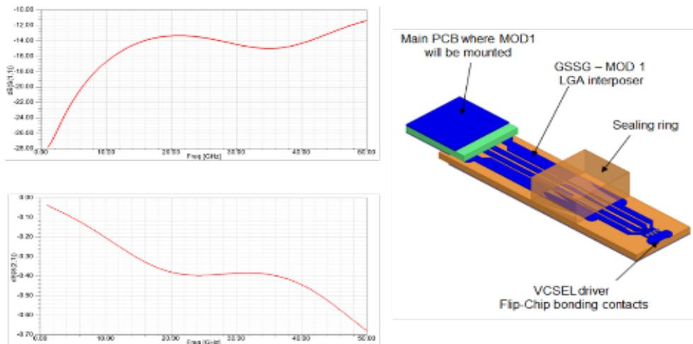
Figure 21. Simulated Return and Insertion Loss of the GSSG lines.
