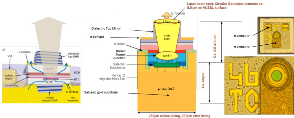
Figure 13 Cross section of the short-cavity VCSEL optimized for high modulation bandwidth.
