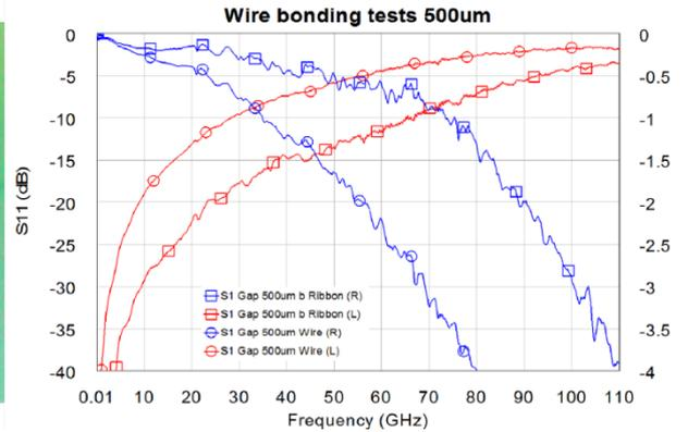
Figure 22 S-parameters of 500 $\mu$ m Wire Bonding loops and 150 $\mu$ m air-gap have been modelled and measured.
