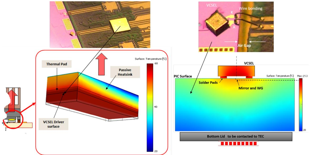
Figure 18. Temperature gradient between the bottom side of the PIC and the VCSEL DBR region for the VCSEL bonded on a PIC, achieved by COMSOL.
