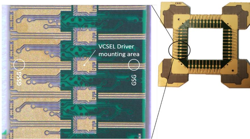
Figure 20. Overview of the Interposer's RF routing lines with 100-Ohm Differential Ground-Signal-Signal-Ground (GSSG) CPW for the VCSEL driver input side and a 50-Ohm GSG CPW toward the VCSEL wire bonding pads.
