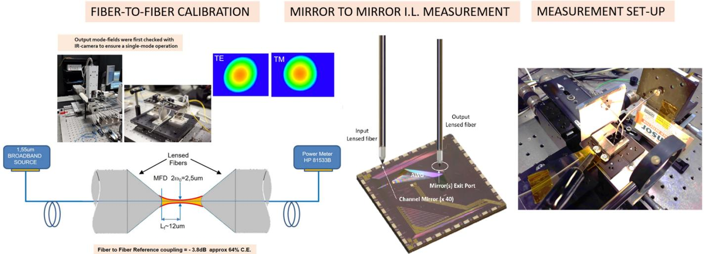
Figure 10 Up-reflecting mirror characterization setup.
