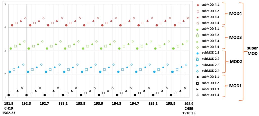
Figure 2. Grid of the VCSEL emission wavelengths for the 4 Tx MODs constituting the PASSION super-MOD.
