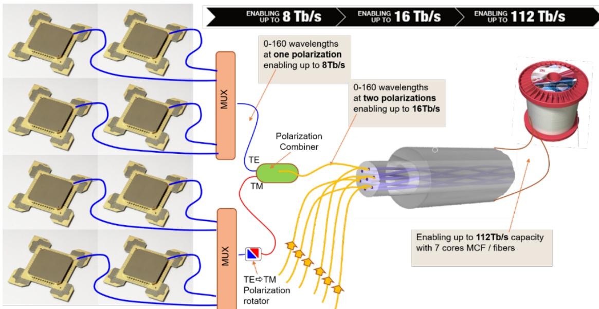
Figure 1. PASSION Tx modular approach for capacity aggregation exploiting spectral, polarization and space dimensions.
