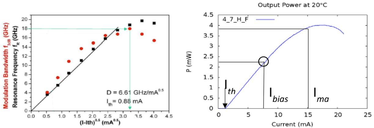
Figure 14 Modulation bandwidth (red circle) and resonance frequency (black square) as a function of the  $I_{\text{bias}}$ . Maximum bandwidth is achieved at  $I_{\text{bias}}$  of about 8 mA, corresponding to  $(I - I_{\text{th}})^{0.5} = 2.64$  ( $I_{\text{th}} = 1 \text{ mA}$ ).
