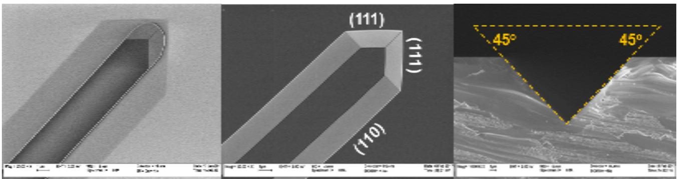
Figure 8 Wet etched mirror 45 degree tilted mirror planes (110) in silicon. Left: with oxide mask on. Middle: after removal of the oxide mask. Right: SEM image of the cross-section of a narrow etched groove with 45 degree tilted mirror planes.
