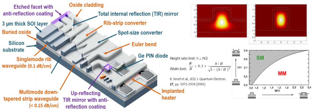
Figure 3. Schematic illustration of the 3 μm SOI platform with rib and strip waveguides, an adiabatic rib-strip converter, spot-size converter, horizontal and vertical total internal reflection (TIR) mirrors and compact Euler bends.
