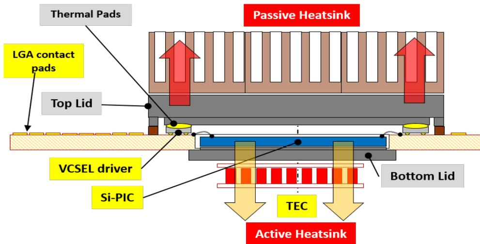
Figure 17 Thermal Model with 2 separate thermal paths.
