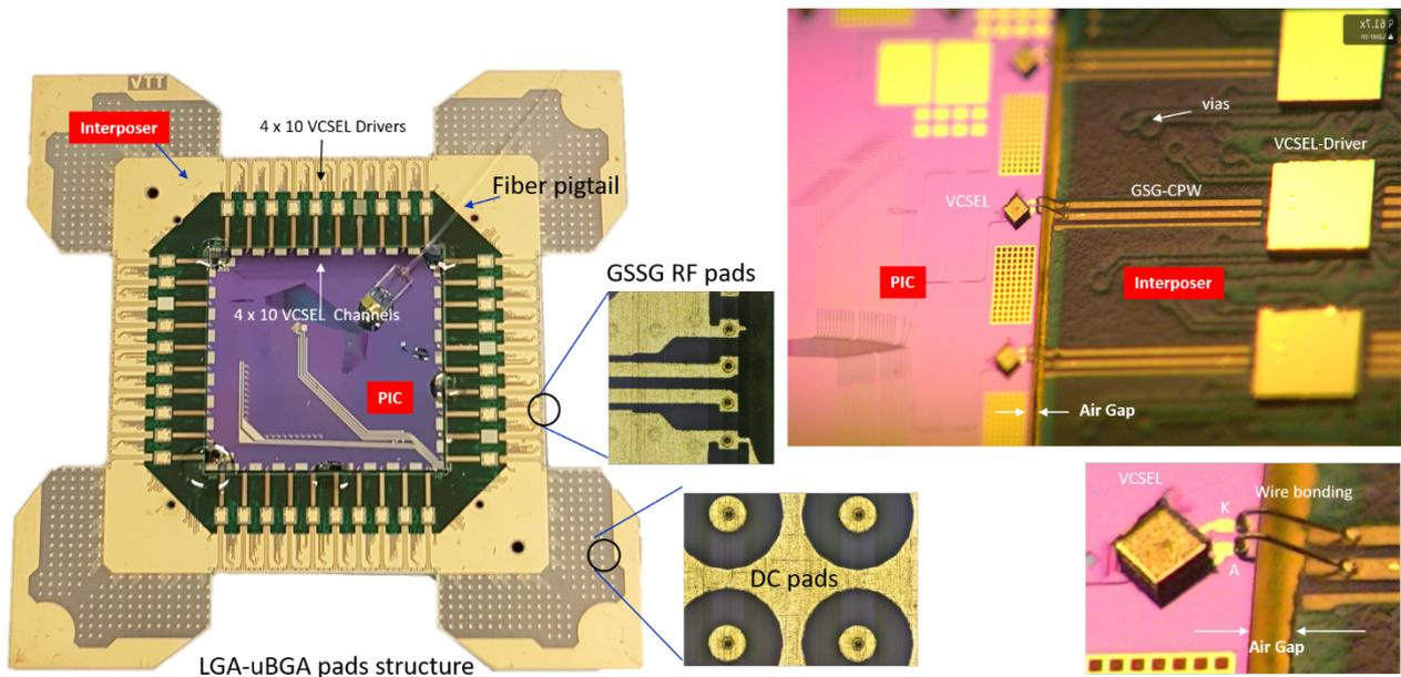
Figure 16. Tx MOD integration scheme: integration of VCSELs and drivers on a 20x20 mm<sup>2</sup> PIC (left). VCSEL flipchip bonded and interconnected (wire-bonding) to Interposer (right). A precise air gap is observed to thermally decouple PIC since working at constant temperature from heat generated by VCSEL Drivers.
