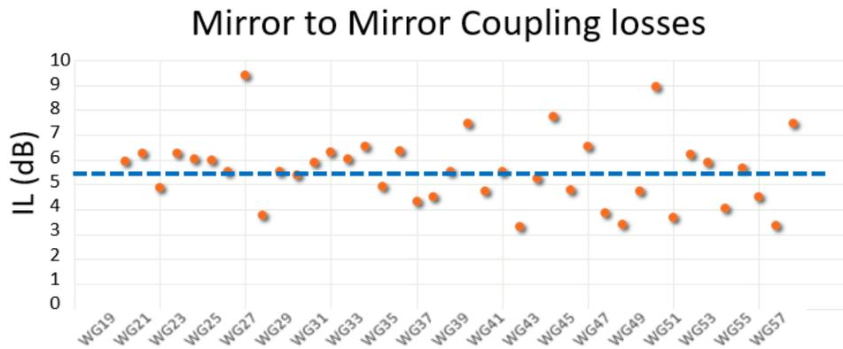
Figure 11 Plots for coupling loss analysis of the up-reflecting mirrors.
