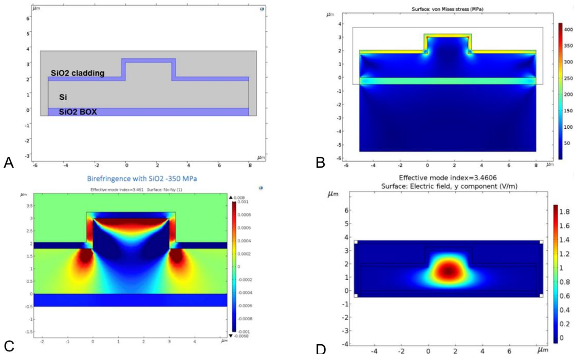
Figure 7. A: An example of a 3  $\mu\text{m}$  rib SOI waveguide with 0.5  $\mu\text{m}$  SiO<sub>2</sub> buried oxide (BOX) layer and 250 nm SiO<sub>2</sub> thermal oxide cladding. B: Simulated material stress profile with -350 MPa compressive stress in the oxide cladding (from literature) and -250 MPa compressive stress in the BOX. C: Modelled waveguide birefringence based on the stress profile in B. D: Simulated optical waveguide mode for TE.
