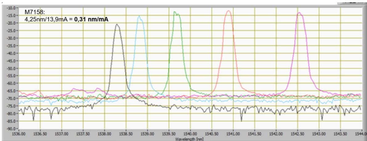
Figure 15 C-Band VCSEL emission tuning by means of the bias current.
