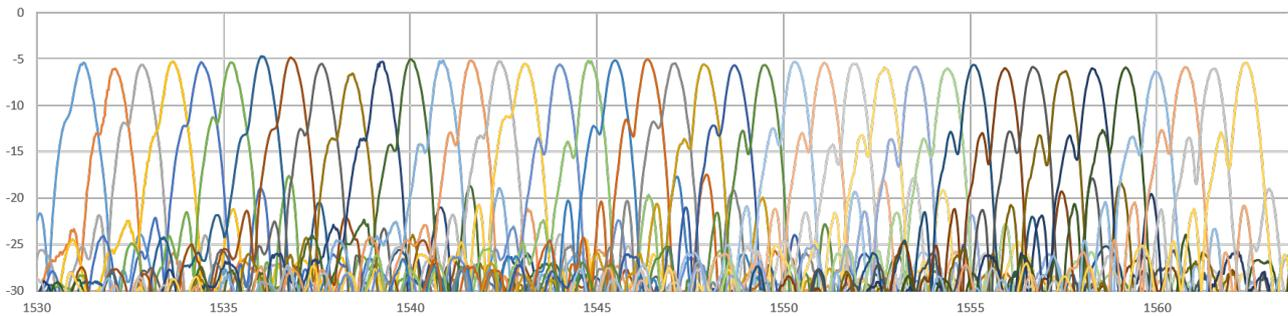
Figure 5 Characterization of 1x40, 100 GHz AWG.
