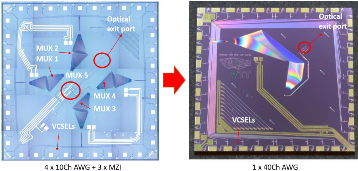
Figure 4 PIC design evolution to the new 40Ch AWG MUX.
