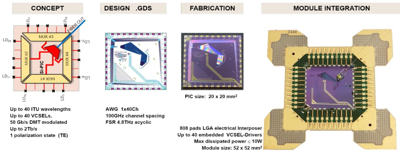
Figure 12. PIC from concept to fabrication and integration in the Tx MOD.
