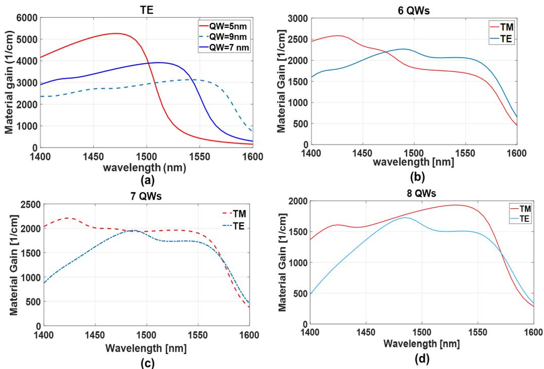
Figure 10 (a) Material gain for TE for 7 QWs with thickness of 5 nm, 7 nm, 9 nm (b) Material gain for TE and TM with 6QW (c) Material gain for TE and TM for 7QW (d) Material gain for TE and TM for 8QW
