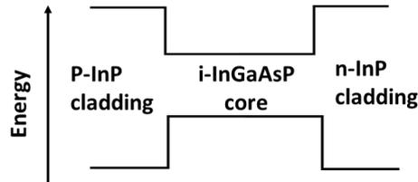
Figure 3 Energy state of a bulk SOA
