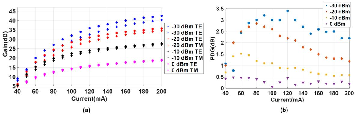
Figure.14 (a) Gain of bulk SOA (dB) vs current (mA) for input powers of -30,-20, -10, 0 dBm
