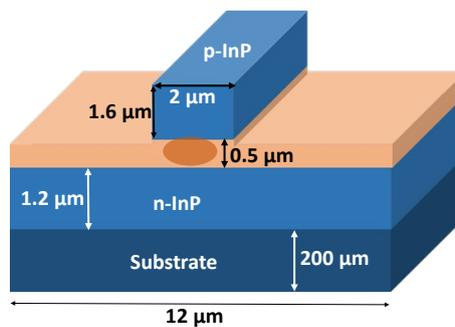
Figure 8 Simulated ridge waveguide structure of an SOA
