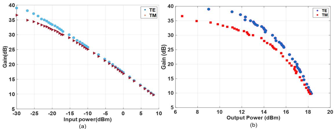
Figure15 Gain of the bulk SOA with respect to (a) input power (dBm) (b) output power (dBm)
