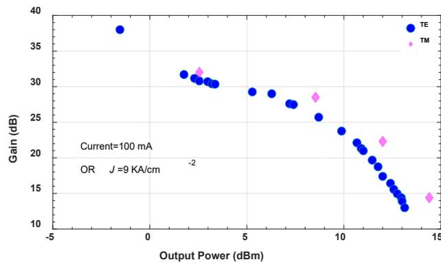
Figure 11 Gain vs output power of a strained MQW SOA, at 100mA injection current for TE and TM polarizations
