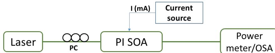
Figure 16 Measurement setup of polarization independent SOAs
