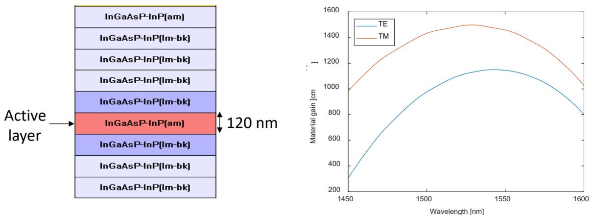
Figure 13 (a) Layer stack of bulk SOA active region (b) Material gain for TE and (c) TM in a bulk SOA
