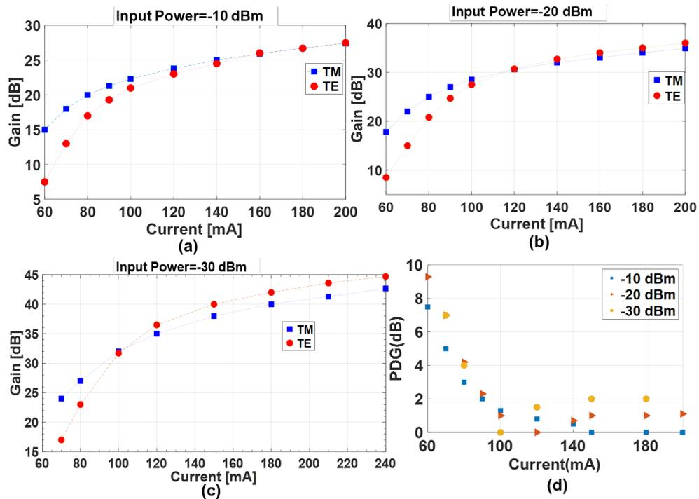
Figure 12 Gain vs current for TM and TE polarizations at input power of (a) -10 dBm (b) -20 dBm (c) -30 dBm (d) PDG comparison
