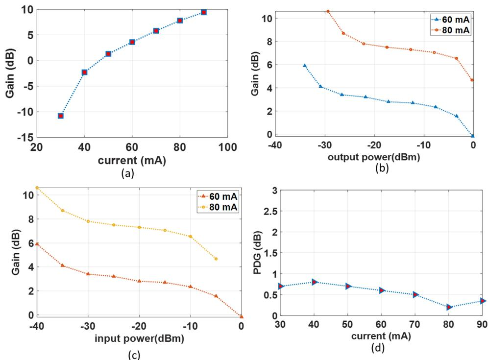
Figure 17 Measurement setup of polarization independent SOA-1 (500  $\mu\text{m}$ ) (a) Gain vs current at input power of -30 dBm, (b) Gain vs output power for bias current of 60 mA and 80 mA (c) Gain vs input power for bias current of 60 mA and 80 mA (d) PDG vs bias current at input power of -25 dBm
