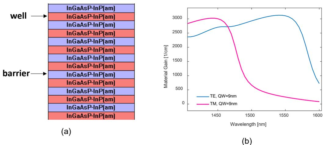
Figure 9 (a) Layer stack of the active region of 7 QW SOA (b) Material gain (TE/TM) for QW=9nm, 7 QWs
