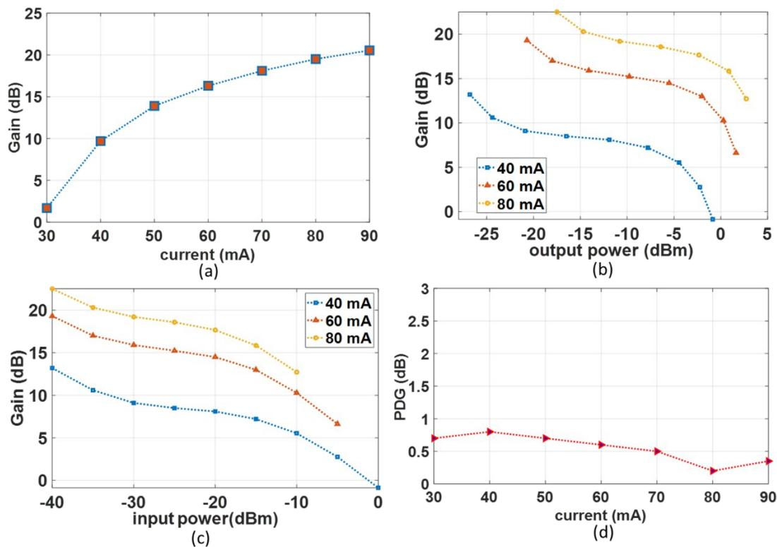
Figure 18 Measurement setup of polarization independent SOA-2 (800  $\mu$ m) SOAs a) Gain vs current at input power of -30 dBm, (b) Gain vs output power for bias current of 60 mA and 80 mA (c) Gain vs input power for bias current of 60 mA and 80 mA (d) polarization dependent gain (PDG) vs bias current at input power of -25 dBm
