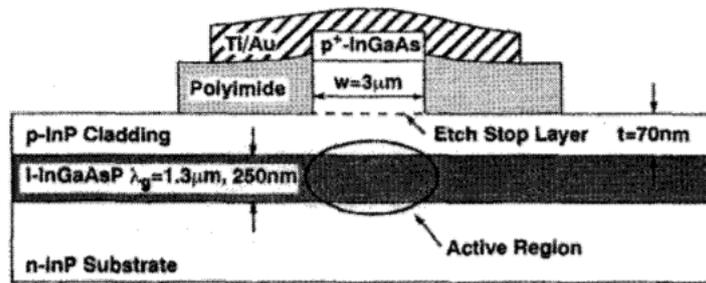
Figure 6 Cross-sectional view of the unstrained bulk PI SOA which requires single step grow [11]
