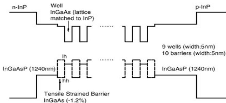
Figure 7 Cross sectional view of the polarization insensitive ridge SOA which requires single step grow [13]
