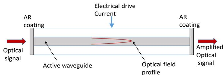
Figure 2 Semiconductor optical amplifier (SOA) basic structure
