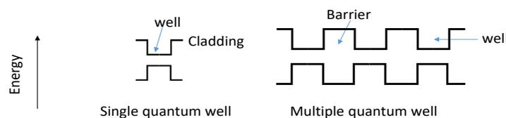
Figure 4 Single quantum well (SQW), Multiple quantum well (MQW) SOAs
