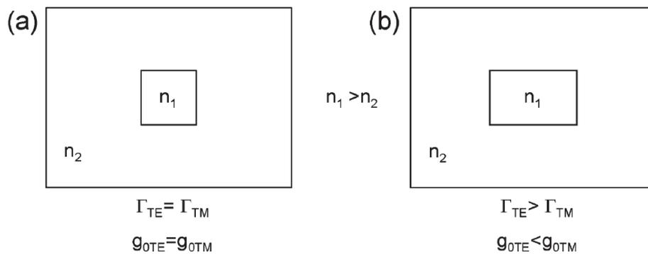
Figure 5 Two schemes for achieving polarization insensitivity, a) square shape structure for which the confinement factor and the material gain are equal, b) rectangular shape waveguide, the material gain compensates the confinement factor imbalance [3]
