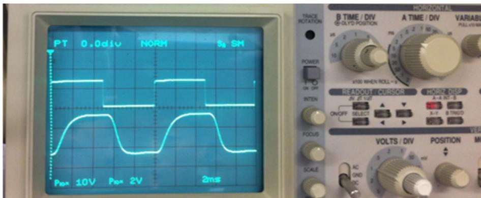
Figure 8. Switching time measurement
