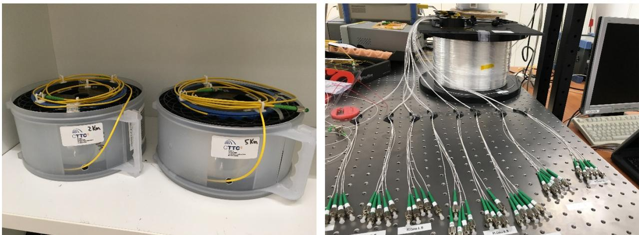
Figure 18 (Left) examples of SMF fibre spools available within the EOS platform. (Right) 19-core fibre of 25 km including fan-in, fan-out elements.
