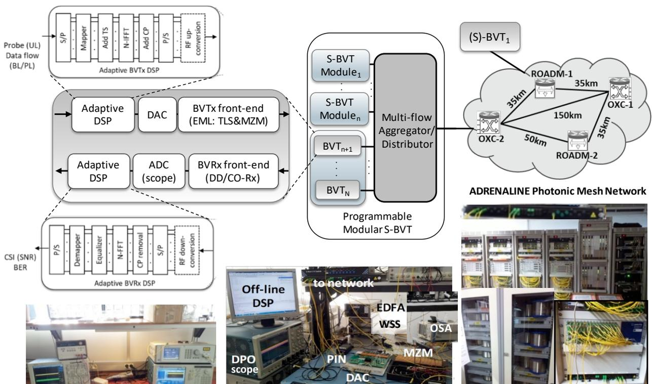
Figure 16 EOS experimental platform (schematic, pictures and examples of DSP and set-ups) and 4-node ADRENALINE testbed network with amplified bidirectional links.
