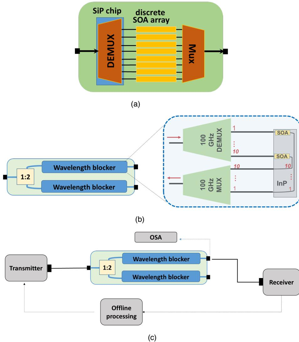
Figure 9 Demo setup for (a) wavelength blocker (WBL) with discrete SOA arrays and SiP deMux chip (b) 1x2 agile WSS functionality via a hybrid integration of SiP passives and with InP SOA array (c) experimental setup of hybrid integrated 1x2 WSS
