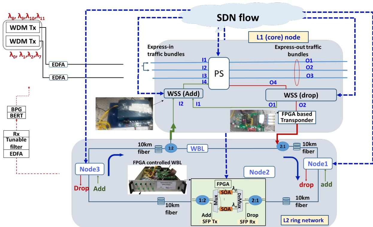
Figure 19. PASSION switching node test bed at Tu/e
