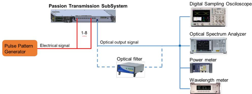
Figure 5. Experimental set-up for Basic Transmission SubSystem validation, characterization and performance evaluation. At SMO R&D Labs VCSELs will be directly modulated by 28 Gb/s NRZ signals while at PoliMI DEIB Lab. they will be modulated by 50 Gb/s DMT signals.
