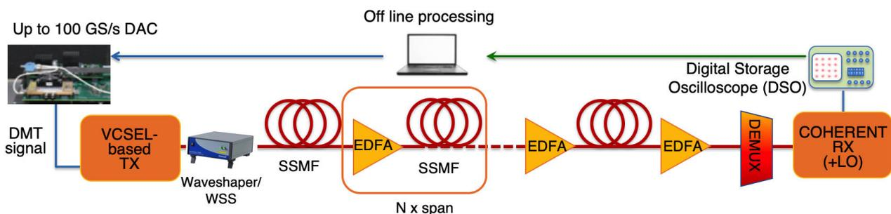
Figure 3. Experimental test bed for multi-span EDFA-amplified transmission performance evaluation, with VCSEL direct modulation (DMT) and coherent detection.
