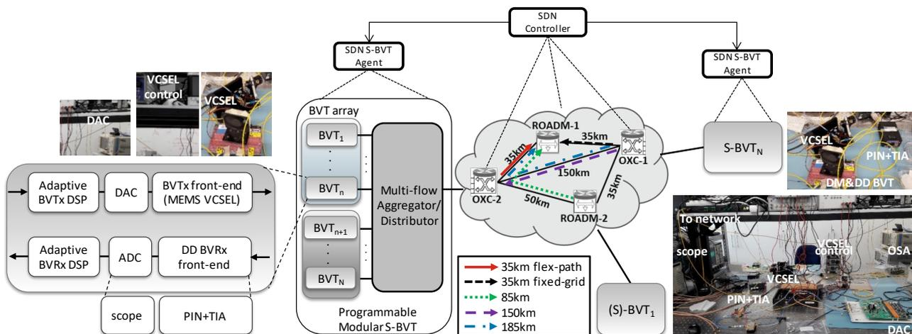
Figure 17 Schematic, set-up and pictures of the SDN-enabled S-BVT adopting MEMS VCSEL at the BVTx front-end. The ADRENALINE network paths considered in the experiment are indicated.
