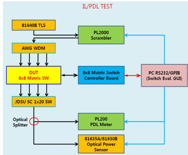
Figure 7. Measurement setup for IL/PDL
