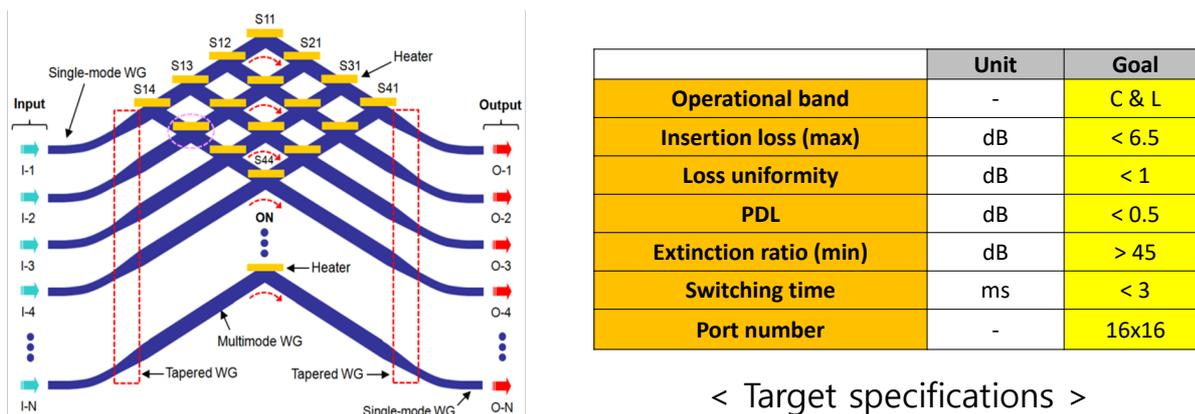
Figure 6. NxN optical matrix switch configuration and (b) target specifications
