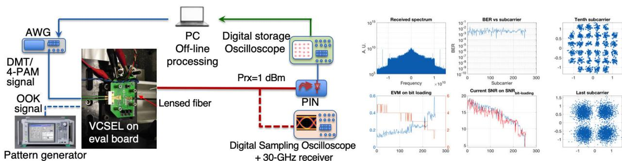
Figure 4. Demo test environment setup (left) and preliminary experimental results with DSB DMT (right)
