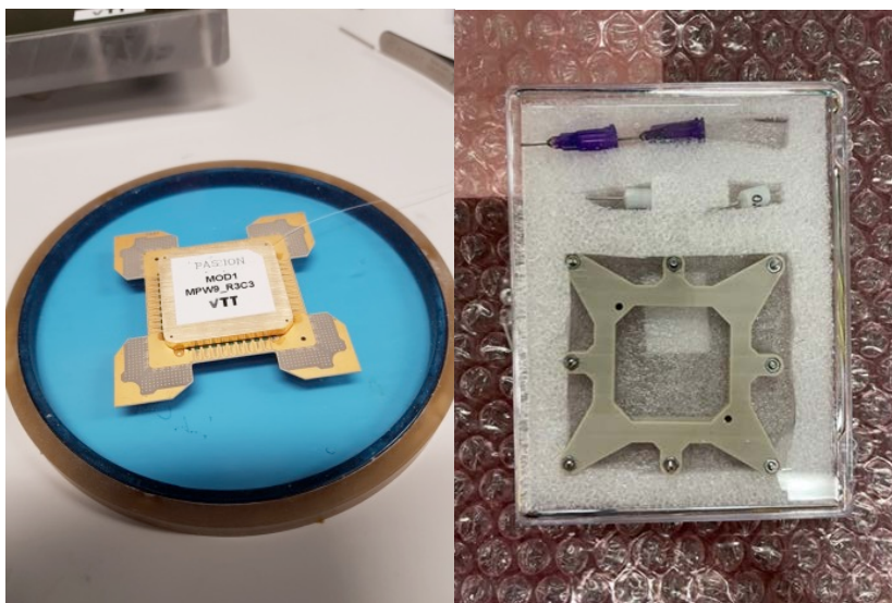
Figure 16. VTT 2-Tb/s TX module and related mechanical clamps.
