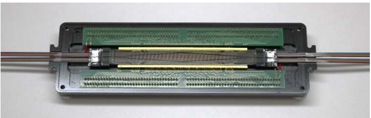
Figure 43. The prototype of 16x16 matrix switch module.
