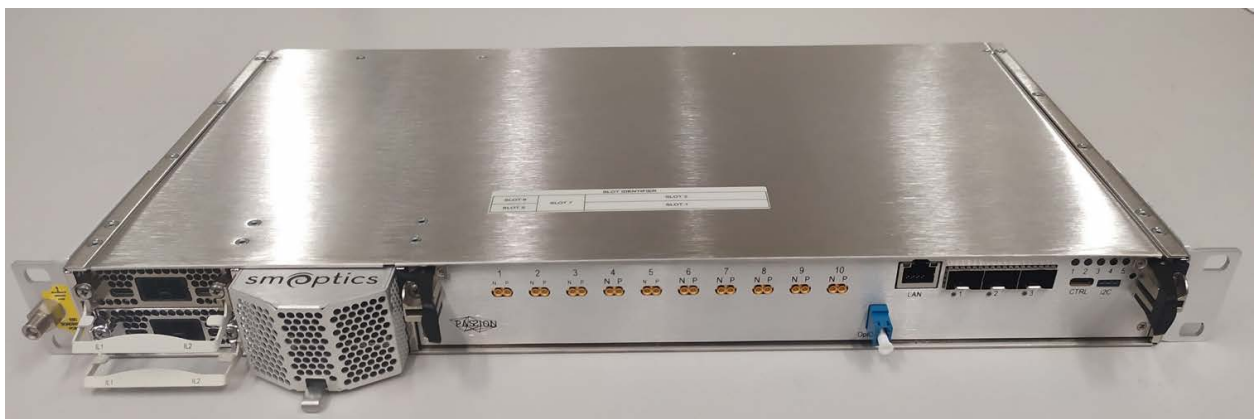
Figure 19. Final 2-Tb/s transmitter board integrated in the ETSI 300mm Subrack.
