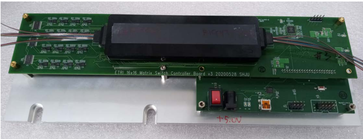
Figure 49. 16x16 polymer matrix switch monted on the controller board.
