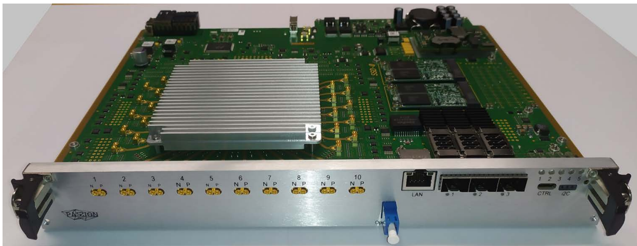
Figure 18. Top view of the final 2-Tb/s transmitter board
