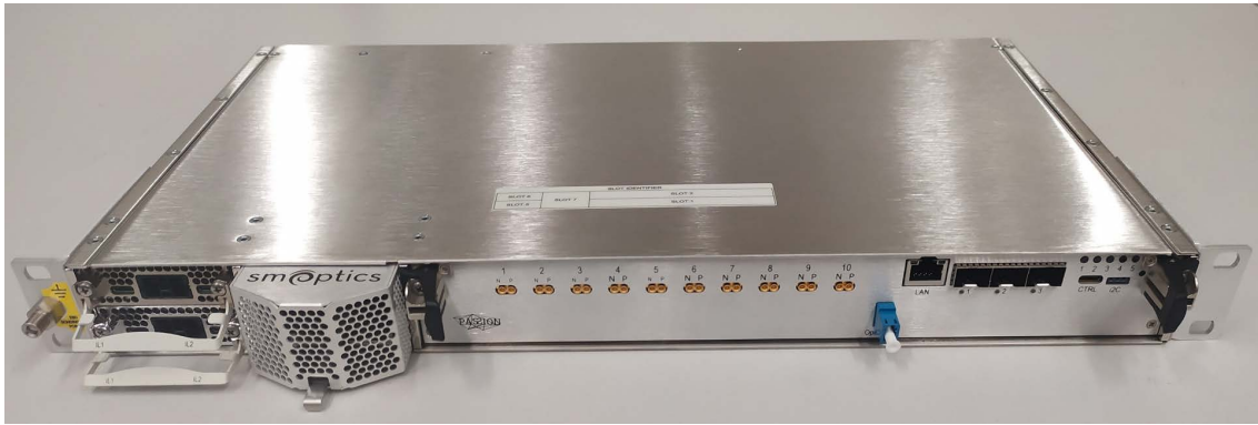
Figure 4 Final 2-Tb/s transmitter board integrated in the ETSI 300mm subrack.
