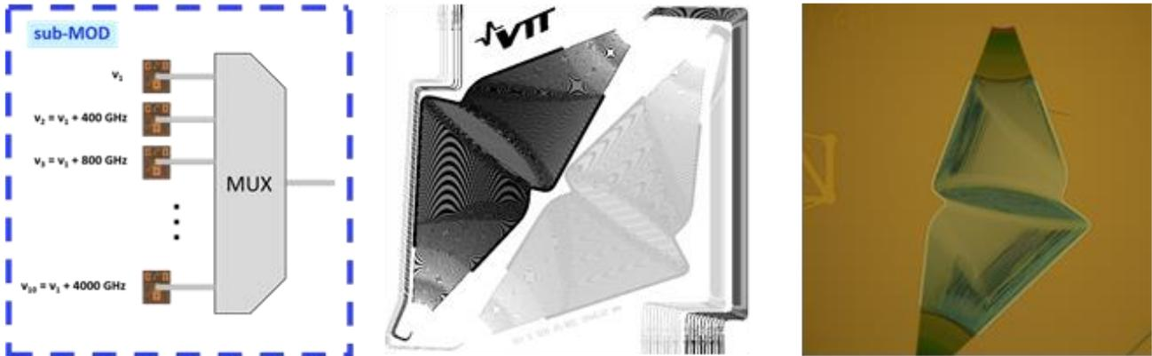
Figure 19 Schematic design (left) and mask design (right) of an S-type 10 channel AWG sub-MOD MUX design with a channel spacing of 400 GHz.
