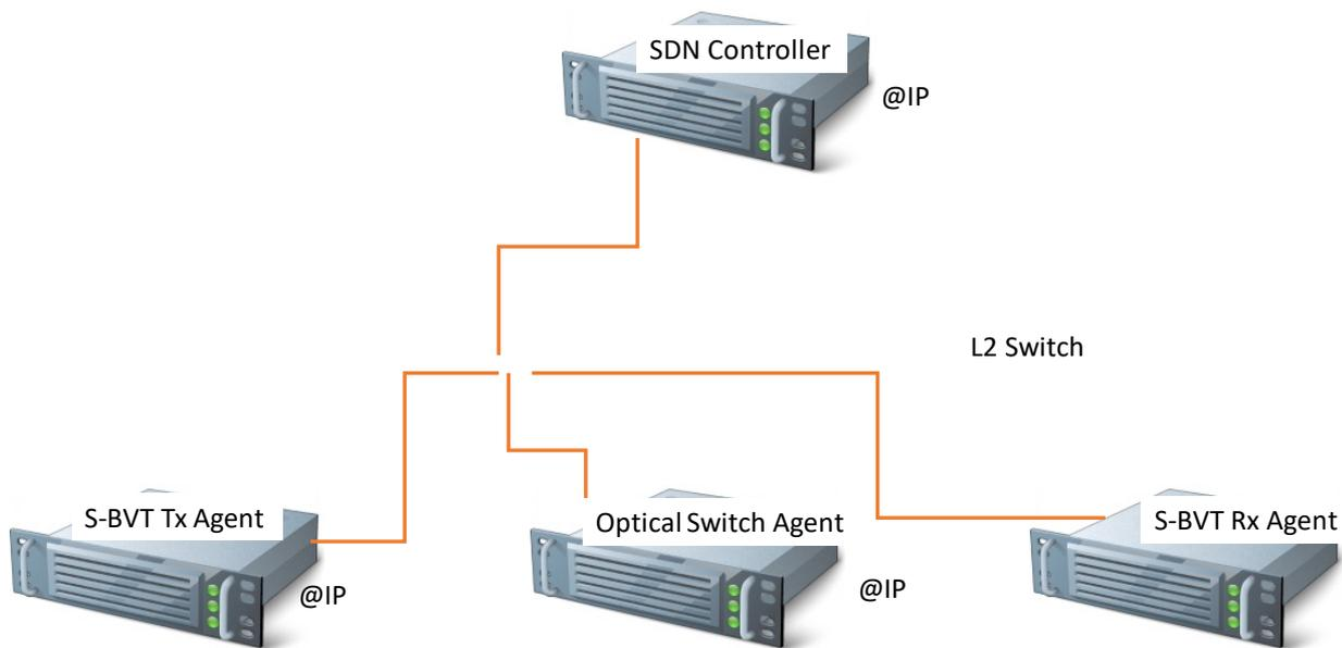
Figure 15 Preliminary validation of the SDN controller functions and data models tailored to the PASSION architecture when automatically setting up an end-to-end optical connection
