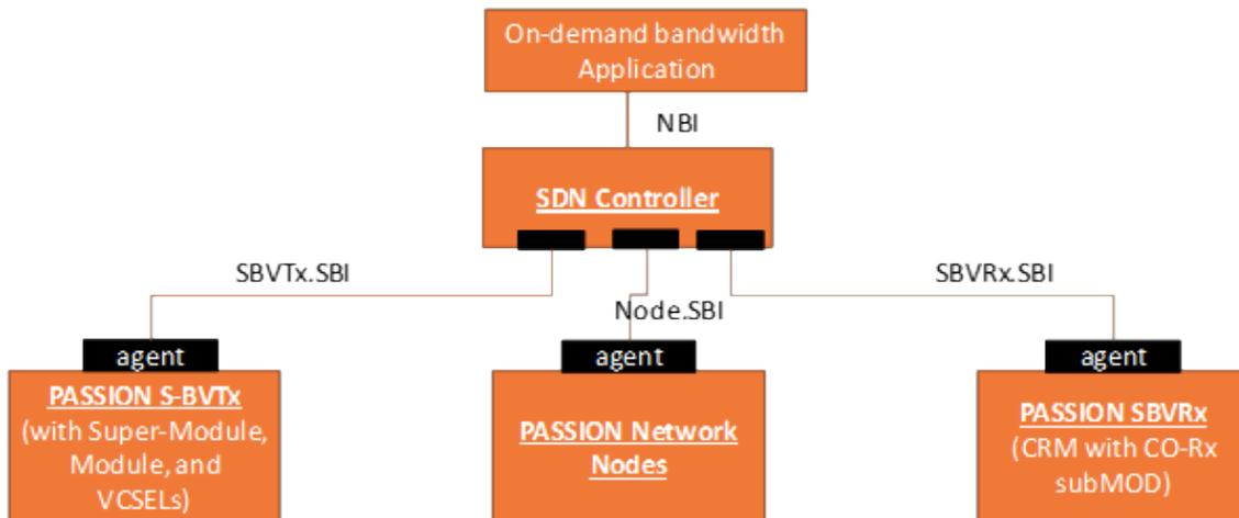
Figure 13 SDN Controller interactions adopted in PASSION (described in MS4 [MS4])
